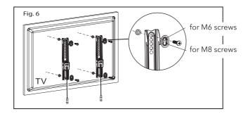
• If you are using the longer screws on a TV with a curved or recessed back, you may also need to use the spacers (D). Use one spacer or two spacers stacked as needed. **Only use** a spacer if necessary
