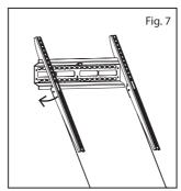
**IMPORTANT!** Verify that both arms are locked to the wall plate. For safety reasons, this mount CANNOT be used unless both arms are securely locked.
