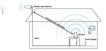
Cottage boosters amplify the available outside cellular signal and distribute it inside the building. To boost signal indoors, some signal must exist outside. The high-gain yagi antenna captures this existing signal, amplifies it and the booster re-broadcasts enhanced signal inside to all devices. The booster then amplifies outgoing signal back to the cell tower.
