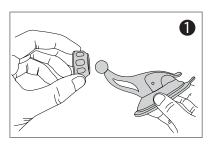
Place the screw cap (threads facing up) over mount's ball joint.
