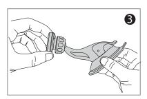
Tighten the screw cap to the cradle by turning it clockwise.
