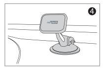
Find a location on your dashboard/windshield that is out of your direct line of sight. Clean the surface on your preferred dashboard/windshield location using the included cleaning wipe. Peel off the wrapping from the bottom of the base and position in place.
