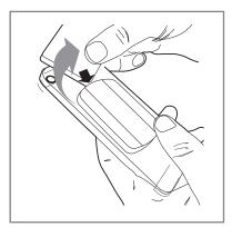
Use a thin plastic card to carefully lift the plate's magnetic surface from the mounting surface. Slowly lift up and remove the plate. Remove adhesive residue with a non-abrasive cleaner.
