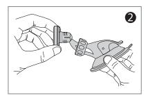
Snap the cradle onto the mount's ball joint, you will hear a "snap" when it is properly connected.
