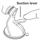
Press down on the base to apply pressure and lock the suction lever.
