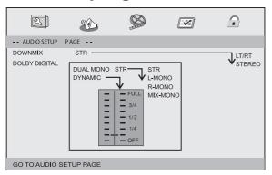
Downmix:This option allows you to set the stereo analog output of your DVD player→ LT/RT:Select this option if your DVD player is connected to a Dolby Pro Logic decoder→ Stereo:Select this option when output delivers sound from only the two front speakers
