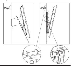
1. Press down on the brackets once it is installed on the wall plate, it will lock in place.
